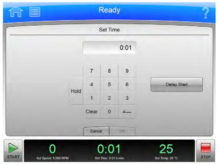
To set the duration for the next run or change the duration of the run in progress, select the **Set Time** Display/Button on the Home Page or the Footer Bar to display the **Set Time** page.
