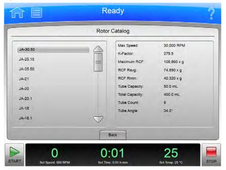
Select the **Rotor Catalog** button on the Menu Page to display the **Rotor Catalog** page. Use this page to examine the detailed specifications for all the rotors compatible with the Avanti JXN series.
