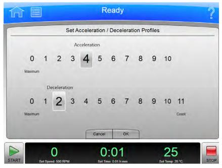
To choose profiles for acceleration and deceleration, select the **Accel/Decel** Display/Button in the Footer Bar of the Home Page to display the **Set Acceleration/Deceleration Profiles** page.
