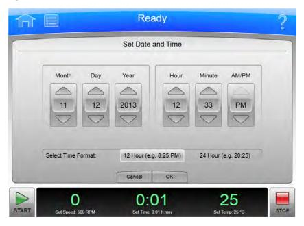
Select the **Set Date and Time** button on System tab of the System Options Page to display the **Set Date and Time** page. Use this page to set the instrument's internal time and date.
