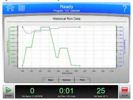
Select the **Run Graph** button on the side menu of the Home Page to display the **Real-Time Run Data** page. This page graphs the current run as it is in progress, or shows the most recent run.
