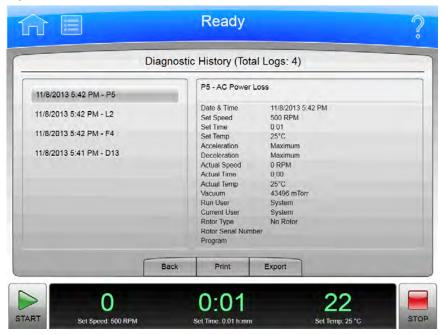
Select the **Diagnostic History** button on the System tab of the System Options Page to display the **Diagnostic History** page. Use this page to review and export the details of incidents that caused a diagnostic message on the instrument (warnings and error messages).
