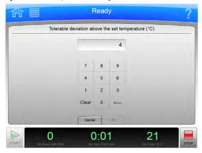
Select the Max Temperature Offset button on the Basic tab of the System Options Page to display the Max Temperature Offset page. Use this page to set the tolerable deviation above the set temperature during a run. Once the tolerable deviation above the set temperature has been selected, the user can specify whether the run should shut down or continue if the overtemp setting is reached by using the Max Temperature Shutdown button on the Basic tab of the System Options Page.
