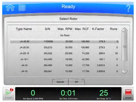
To select a rotor for the next run, select the **Rotor** Display/Button on the Home Page or the **Select Rotor** button on either the Set Speed Page or the Set Speed  $\omega^2 t$  Time Page to display the **Select Rotor** page. This page displays the library of rotors that have been entered for your instrument.
