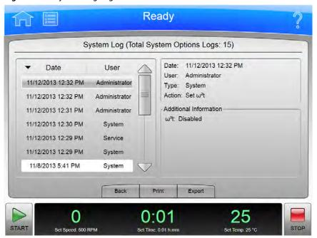
To display the history of changes to the system, select the **System Log** button on the System tab of the **System Options** Page to display the **System Log** page.
