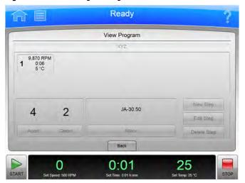
To create a run program, select the **New** button on the Select Program Page to display the **New Program** page. To edit or view a run program, select the program and select the **Edit** or **View** button on the Select Program Page to display the **Edit Program or View Program** page. The pages are identical except for which buttons are active. (The **View Program** page does not permit editing.)
