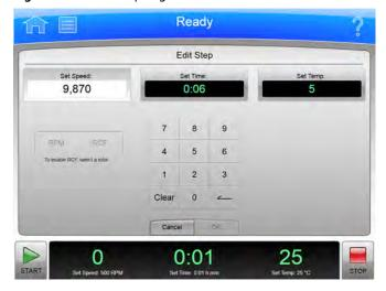
To create a step within a run program, select the **New Step** button on the New Program Page or the Edit Program Page to display the **New Step** page. To edit a step within a run program, select the step and select the **Edit Step** button on the New Program Page or the Edit Program Page to display the **Edit Step** page. The pages contain the same options.
