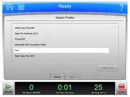
To select a printer for the system, select the **Select Printer** button on the Network tab of the System Options Page to display the Select Printer page.
