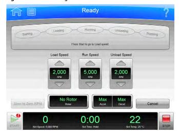
When the rotor reaches the Loading speed, the status display highlights Loading, to show that you have moved into the next phase.
