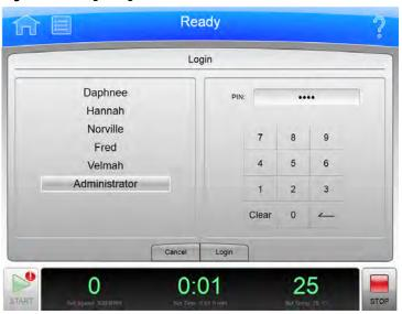
If the user login requirement has been enabled for the instrument, you must log in to the system use it. Select the Login button on the Home Page to display the Login page.
