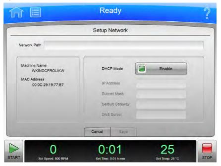
Select the **Setup Network** button on Network tab of the **System Options** Page to display the **Setup Network** page. Use this page to configure the network connection.
