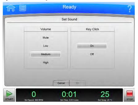
Select the **Set Sound** button on the System tab of the System Options Page to display the **Set Sound** page. Use this page to set the volume and enable or disable the key click option.
