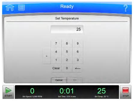
To set the temperature for the next run or change the temperature for the run in progress, select the **Set Temperature** button on the Home Page or the Footer Bar to display the **Set Temperature** page.
