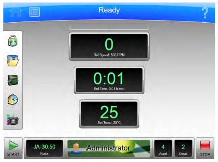
The **Home** page is the first operational page to appear after the instrument startup. To display the Home page, select the **Home** page button on the Header Bar. It is the basic page from which you begin most operations. The large fields are designed for viewing from a distance.
