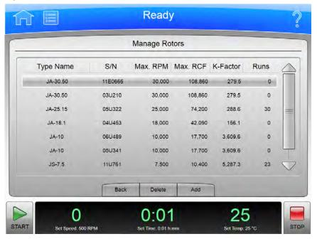
To add or delete rotors from your rotor library, select the **Manage Rotors** button on the System tab of the System Options Page to display the **Manage Rotors** page. See Managing Rotors for more information.
