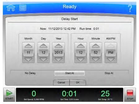
To set a future start or end time for the next run, select the **Delay Start** button on the Set Time Page or the Set Speed  $\omega^2 t$  Time Page to display the **Delay Start** page.
