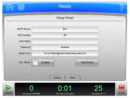
Select the **Setup Email** button on the Network tab of the **System Options Page** to display the **Setup Email** page. Use this page to configure settings for email sent from the instrument. When email is configured, the instrument sends diagnostic notifications to all users with email addresses defined in their user profiles.
