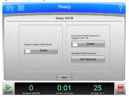
Select the Setup VNC button on the Network tab of the System Options Page to display the **Setup VNC** page. Use this page to connect to the instrument from a laptop or other remote device.
